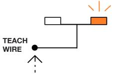
ACCORDING TO CONFIGURATION OUTPUT (PNP/NPN) HOLD TEACH WIRE FOR 8 SECONDS TO SWITCH FROM NO TO NC CONFIGURATION
