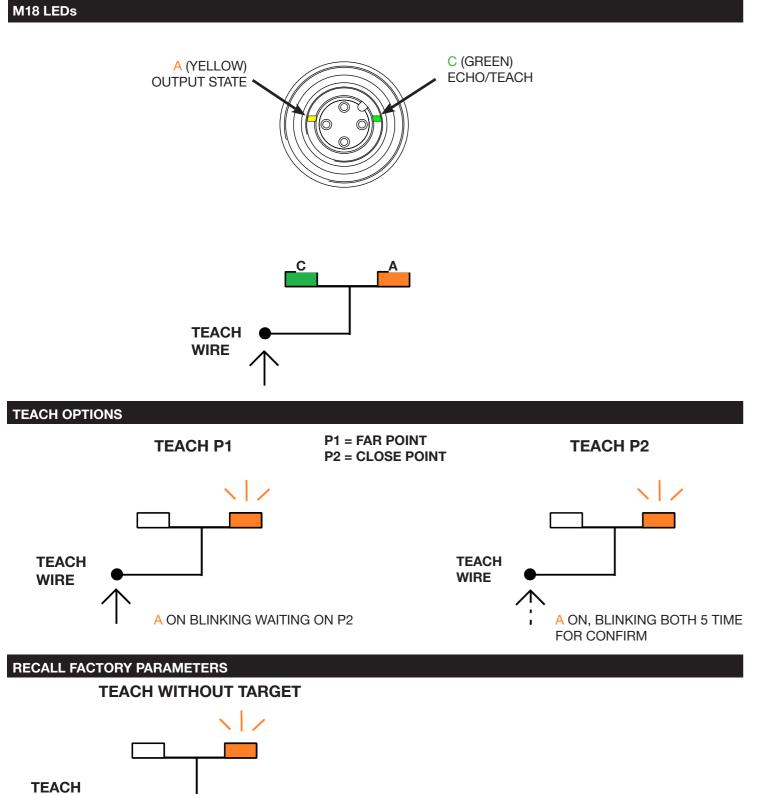
A ON, BLINKING BOTH 5 TIME FOR CONFIRM
