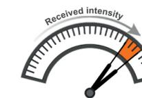
UV light intensity is greatly reduced by transparent material, resulting in important received light intensity loss when a transparent object is in the light path. This makes detection extremely reliable and adjustment easy. With conventional technology, light intensity is only slightly reduced by transparent material. Fine adjustment is critical and detection can be unreliable with difficult materials and applications.
