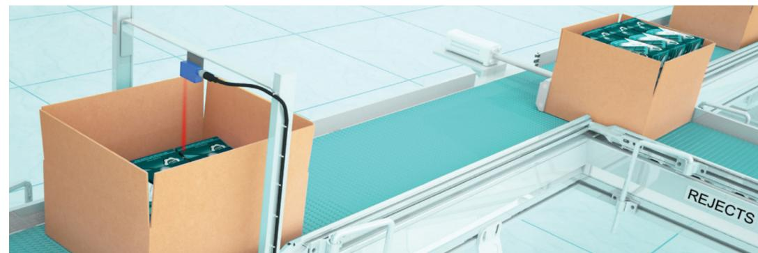
In a packaging application, the flexible mounting system of C23 sensors ensures easy installation. A background suppression type with teach function, mounted above the conveyor belt, provides highly reliable sensing. Its simple one- or two-step teach procedure optimizes initial sensor set-up. Sensing range is adjustable either via the teach button or via IO-Link. The IO-Link interface also allows stored sensitivity parameters to be updated remotely, without manual intervention.
