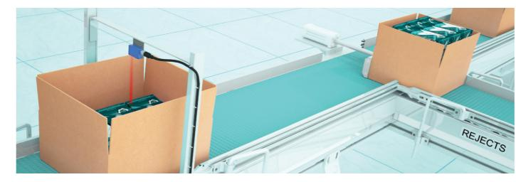
In a packaging application, the flexible mounting system of C23 sensors ensures easy installation. A background suppression type with teach function, mounted above the conveyor belt, provides highly reliable sensing. Its simple one- or two-step teach procedure optimizes initial sensor set-up. Sensing range is adjustable either via the teach button or via IO-Link. The IO-Link interface also allows stored sensitivity parameters to be updated remotely, without manual intervention.
