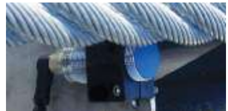
Distance monitoring for position control
