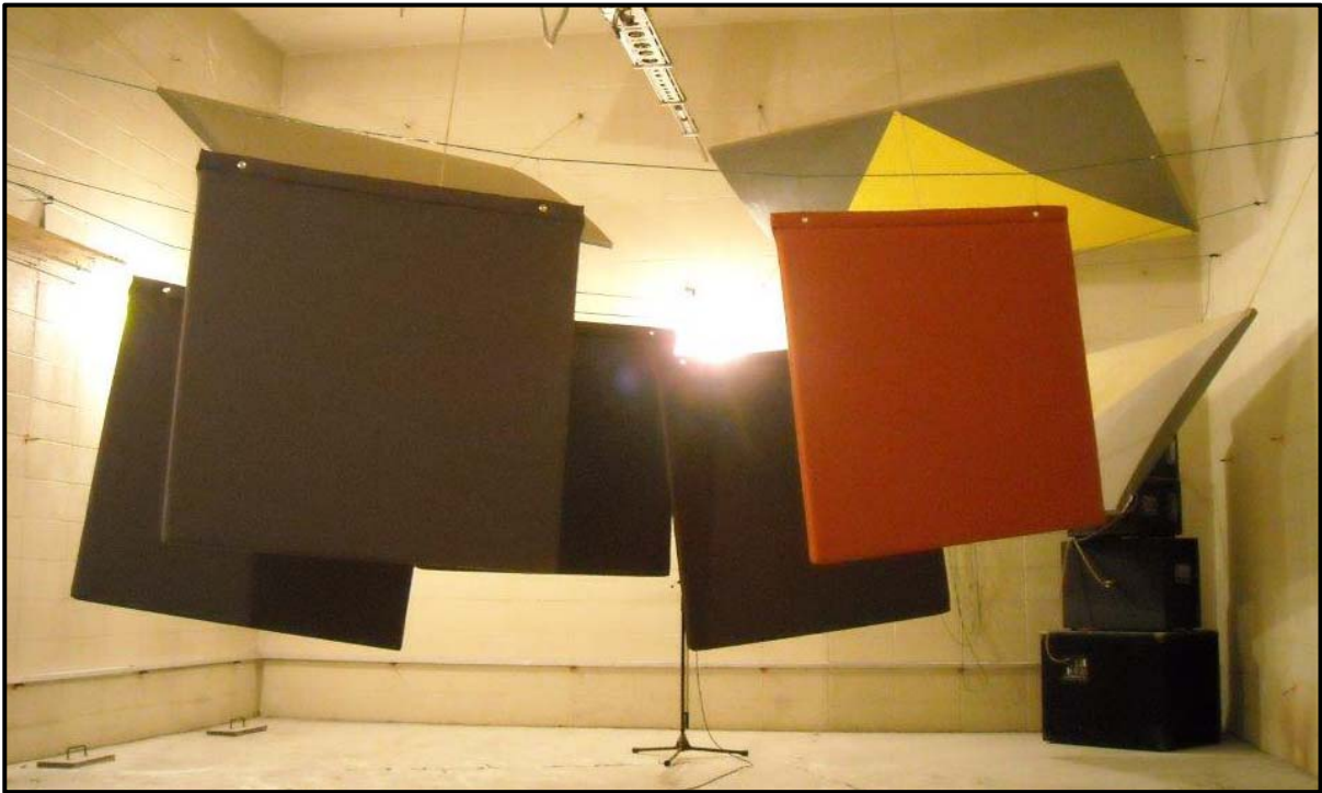
Figure 2 – Specimen Set Up For Fabric-Wrapped Baffles
