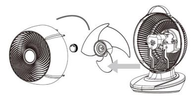
3. Clean the fan blades and the internal part of the fan using a soft dry cloth. Reverse the procedure to put the fan back together. Make sure the locking cap is tightened securely.
