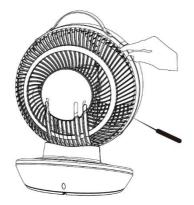
2. Squeeze four locks to pull away the front guard. At the front of the fan blades there is a locking cap – unscrew the cap in a clockwise motion to remove the fan blades.
