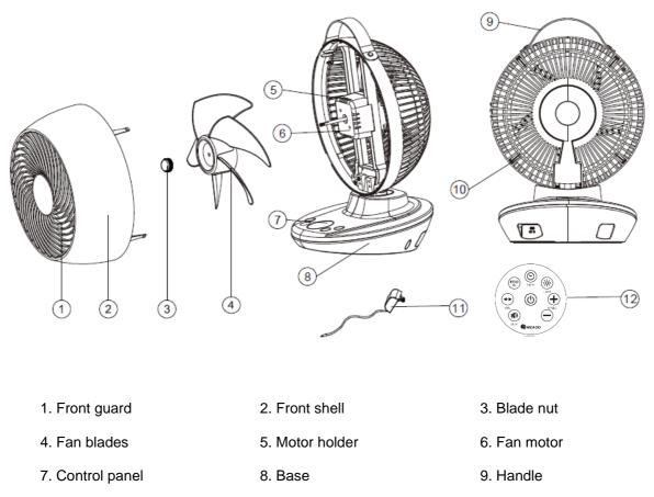
10. Back guard 11. Cable and mains adapter 12. Remote control
