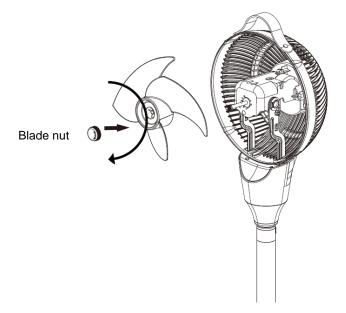
3. Clean the fan blades and the internal part of the fan using a soft dry cloth. Reverse the procedure to put the air circulator back together. Make sure the locking cap is tightened securely.
