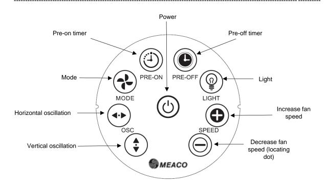
The following functions are only available via the remote control. All other buttons on the remote-control work in the same way as the control panel (see pages 4 and 5). The remote control has a range of approximately three metres. Before using the remote control, remove the plastic tab.
