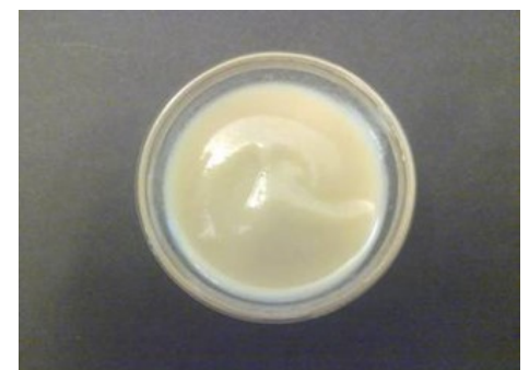
Oat ® COM created a margarine-like emulsion, when first mixed with oil and then appropriate amount of water. The emulsion was easy to create in cold process. The oil and water fractions did not separate from the emulsion during storage.
