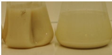
Oat ® COM was mixed in a 5% water suspension and did not settle within 1 hour, when other colloidal oatmeals showed clear signs of settlement.
