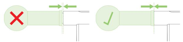
There should be no gap between the grip and the frame, and you shouldn't be able to rotate the grip. If there is a gap, then rotate the grip whilst pushing gently until the gap is closed, and the grip can't turn.
