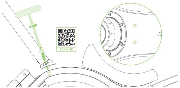
To attach, locate the tiller's end into the tiller mount on the frame. Using the 4mm allen key, secure the tiller to the frame with the bolts provided, tighten to 2.5-3nm.
