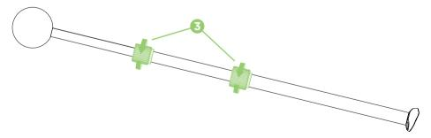
Tighten the twist locks by rotating them in a clockwise direction. Reverse these steps to shorten the tiller.
