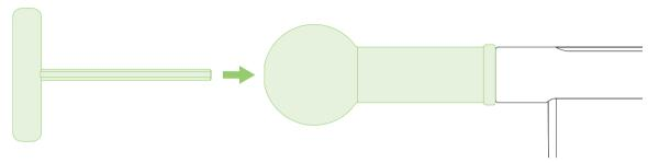
Insert the allen key into the hole at the end of the grip.
