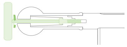
5 Tighten the bolt by turning the allen key clockwise until the bolt is finger tight - this is between 2.5-3Nm. Do not over tighten as this may damage the grip.
