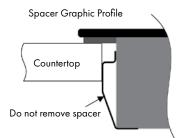
**NOTE**: The cooktops include spacers on both sides to ensure proper airflow once installed. Do not remove the spacers.
