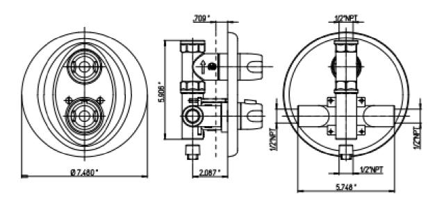
Water Harmony thermostatic valve with ¾" ceramic disk volume control
