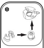
Enclosed are 2 small spiral caps. Before starting assembly combine and insert into bottom.
