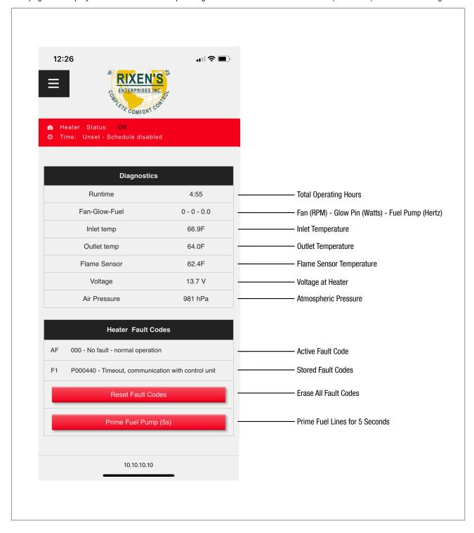
Prime Fuel Pump: This is only useful for initial installation, or when the fuel line to the heater lost its prime (due to maintenance or an empty fuel tank). When selecting this button, the fuel pump will activate for 5 seconds. If in doubt, please do NOT use this function unless directed to do so by a technician.
