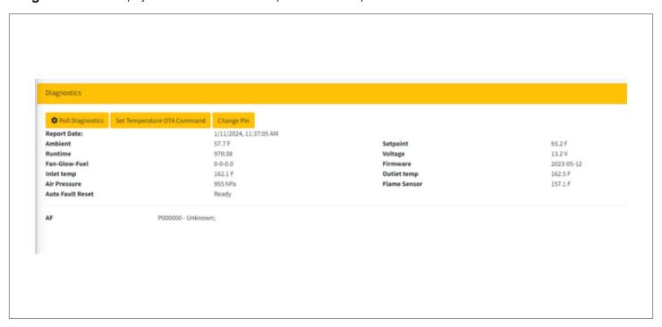
Set Temperature will allow the user, technician, or service center to remotely set the temperature. Note, the RV owner/operator must be present at the RV to manually activate the MCS7 heating system via the touchscreen controller for safety purposes.
