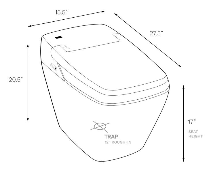
SEAT LENGTH 17" SEAT WIDTH: 15" SEAT OPENING LENGTH: 12.5" SEAT OPENING WIDTH: 8"
