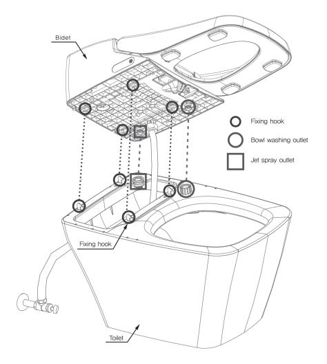
\*Do not use excessive force when attaching the bidet seat to the toilet base.
