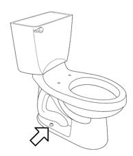
Remove the toilet and wax ring, leaving the exposed trap (pictured below).
