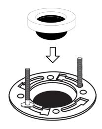
• Line up the toilet base over the flange screws. Place the toilet base and re-secure the flange bolts.
