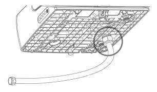
Attach the bidet seat to the toilet base by lining up the mounting hooks and pressing down until you hear a "click".
