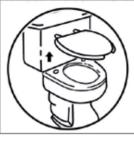
Remove Existing seat and lid. Release the bolts on both side of the existing toilet seat.
