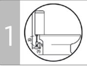
Shut water supply by turning it to the right and disassemble the water hose.
