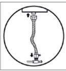
Connect the water supply hose to the supplied T-Valve.
