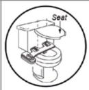
Mount bidet and toilet seat/lid over toilet mounting holes. Supplied rubber O-rings should be placed under the bidet mounting bracket to protect and secure bidet on the toilet.
