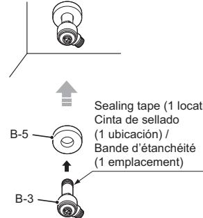
\*Wrap the sealing tape around the threaded part and attach it.
