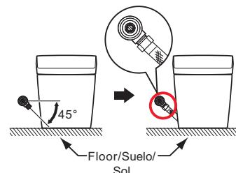
**Shutoff valve installation direction for water supply from the floor /**
