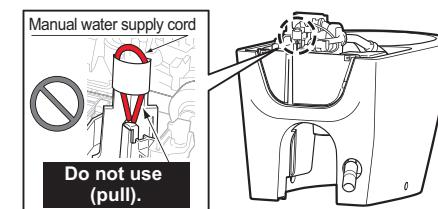
By pulling the manual water supply cord (orange) until it stops, you can toggle the flow of water to the toilet bowl on and off.
