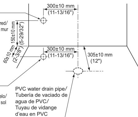
\*If there is a gap between the discharge pipe and floor, fill it with mold-resistant silicone-based seal material (Mediseal). /
