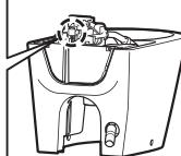
By pulling the manual water supply cord (orange) until it stops, you can toggle the flow of water to the toilet bowl on and off./
