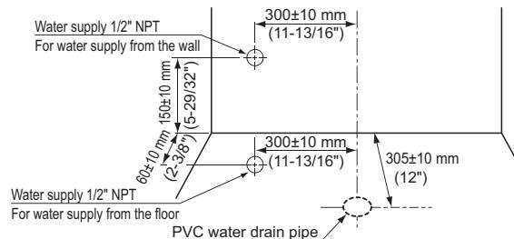
**Caution** The height of the water supply pipe should be within 0+5/8 mm from the floor/wall. The shutoff valve cover may tilt or float and may not be attached.
