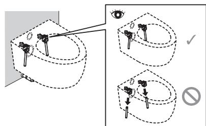
**EN** Use D-1 as support when installing the toilet bowl. Use B-1 to securely fasten A-1 to the wall. Verify that A-1 is level and flat against the wall. Do not remove the guide tubes after installation. Confirm A-1 is securely fastened to wall. Leave no gap. Do not overtighten.
