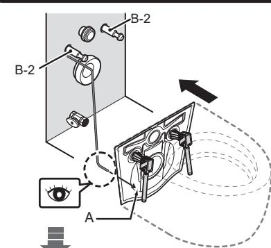
**EN** Note: When placing the toilet bowl, be careful not to pinch the cord. Pass the cord all way inside the bowl.
