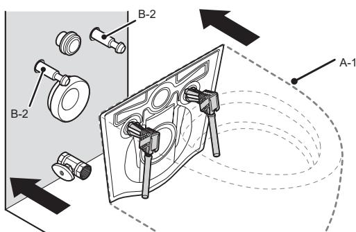
**EN** Align the mounting holes in A-1 with B-2 and press A-1 into the wall. The supply inlet and waste outlet gaskets must fully engage and the back surface of A-1 must be completely flat against the wall. Put support on the underside of the bowl if needed to ensure the back surface of A-1 stays flat against the wall for the rest of the installation.
