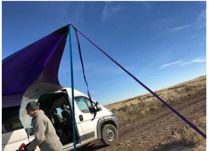
Put the pole together and insert into grommet in the tarp and stand the pole up at an angle
