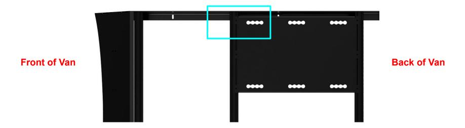
2B - Place the deck panel on the crossbars. Make sure the 6 holes on the deck panels line up with the center of the crossbar channels.
