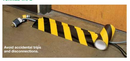
Tunnel Tape is effective for hiding cords and preventing trips. This tape forms a "tunnel" to safely hide wires and cables. Made of durable 0.25mm, laminated polyethylene, this tape has a special adhesive backing that adheres to any surface - even carpeting. Tunnel tape can be hand torn, repositioned several times and will not leave a sticky residue when it is removed - adhesive-free 'tunnel' means no glue on cords.
