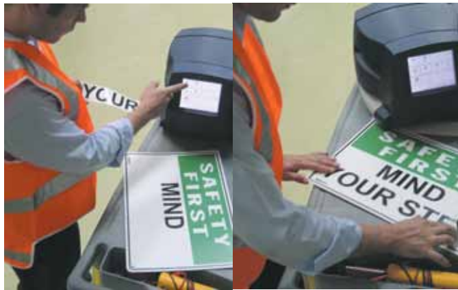
Print text or pictogram | Remove liner | Apply to blank sign panel.
