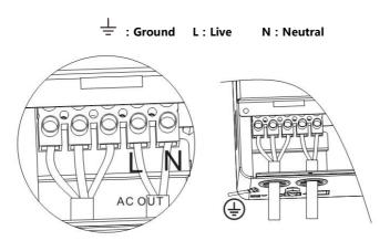
Note: The grounding wire shall be as thick as possible (cross-sectional area is not less than 4mm2). The grounding point shall be as close as possible to the all-in-one solar charge inverter.
