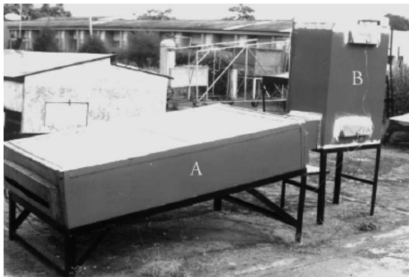
Fig. 9. Photograph of the air heating system. (A) Collector assembly with energy storage and air-heating subsystems; (B) heated space.
