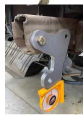
on inside of frame and then lock washers (or loc nuts) and nuts. Torque 5/8 bolts to 100 ft-lbs. Repeat for other side.
