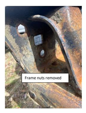
Once frame nuts are removed, remove the 9/16" suspension nut (13/16" wrench size)
