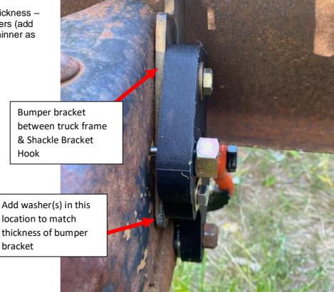
Once correct washer thickness is established, you are ready to bolt Shackle Bracket onto truck
