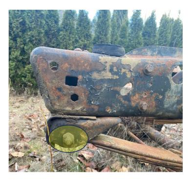
If your truck was equipped with with bumper brackets, you will need to add a washer between the Shackle Bracket Hook and frame to account for the thickness of the bumper bracket. Multiple 9/16" washers are included in our hardware kit for this.
