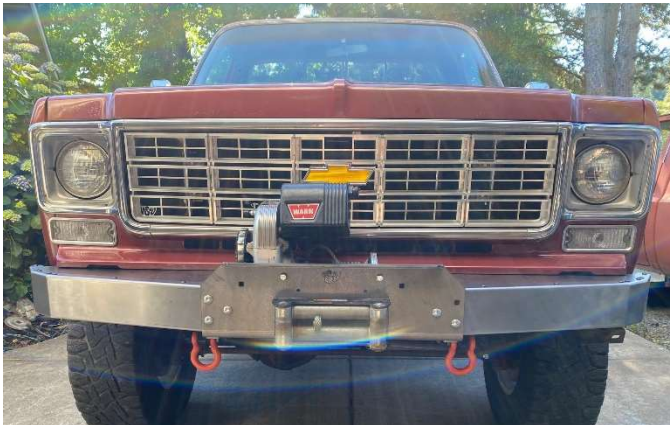
'GOAT' bumper installed on 1977 Chevrolet ¾ ton 4x4 with WARN 8274 winch and Engineered Vintage Shackle Bracket Tow Hooks (sold separately)
