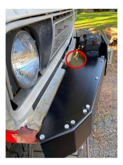
Once tops are installed, install outer bumper braces on frame brackets in bottom rear hole and line up outer holes with outer bumper brace bracket. Bumper bracket can also be installed in different holes if that lines up better with your truck
