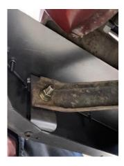
If your winch is a WARN 8200 or 8274, now install the 8274 winch braces on both sides using 7/16 carriage bolts in highlighted locations – tighten these bolts
