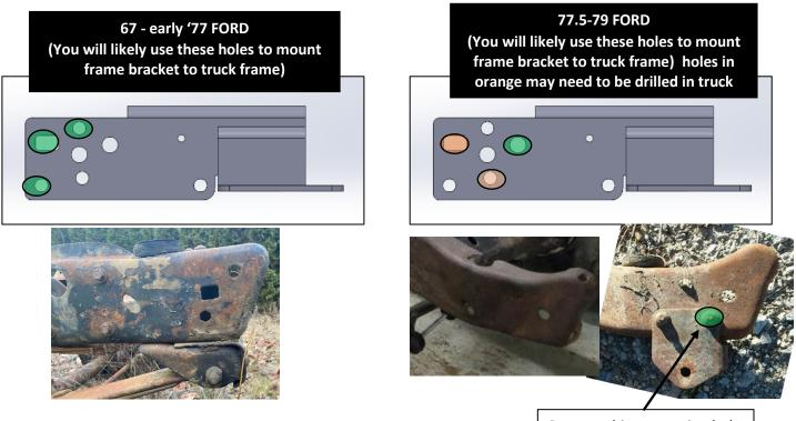
If your truck does not have (3) holes in the frame that correspond to holes in frame bracket, you will need to drill your truck frame.
