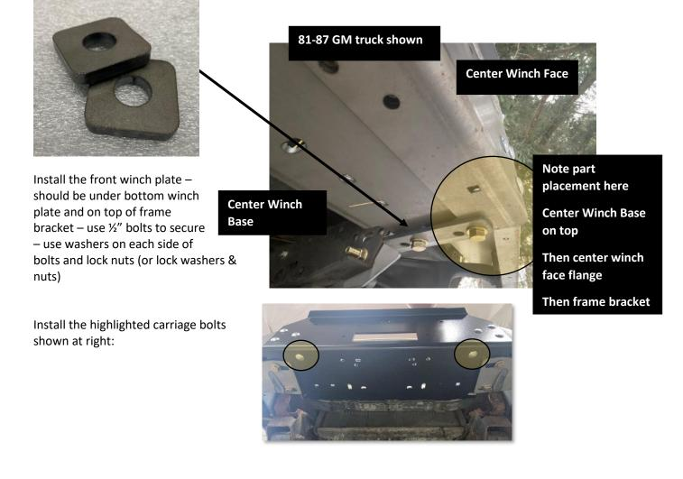
Install the top support plate as shown on both sides (bumper wings will be installed next)
