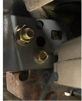
Install outer bumper brace bracket in each bumper wing in appropriate hole that lines up with stock bumper outer brace – this may take some trial & error with bracket to line up. Use a  $\frac{1}{2}$ " bolt to attach 'GOAT' bumper brace to stock outer bumper brace.
