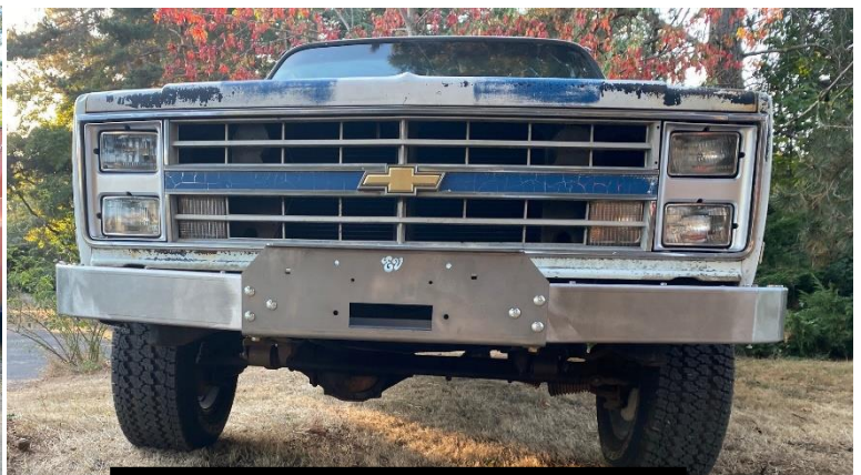
'GOAT' bumper installed on 1987 Chevrolet ¾ ton 4x4
