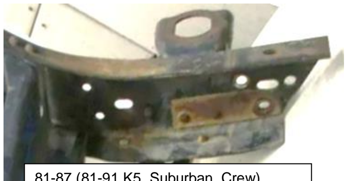
81-87 (81-91 K5, Suburban, Crew) frame rail with tow hook frame reinforcement bracket riveted to frame
