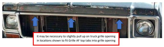
Check alignment of Grille AF in opening of truck – adjust as necessary so it is centered side to side as well as up & down.
