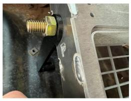
Once bracket is attached to Grille AF, mark location on the core support to drill hole.
