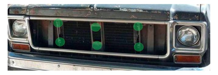
Remove headlight bezels on both sides of truck (5 Phillips head or Torx screws per side)
