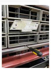
Install new plastic GM mounting tabs in the six locations highlighted below
