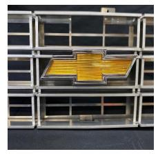
Install grille in truck – the tabs on perimeter of grille are intended for alignment only – not mounting.
