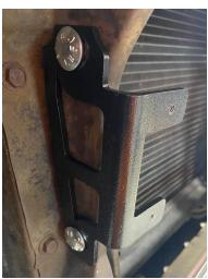
Tighten bolts so that they are snug, but bracket is still able to move slightly to adjust grille in grille opening
