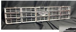
Special note on handling of polished grilles: We recommend handling these with cotton gloves or cotton tshirt during install. Any smudges or light scratches can be cleaned with common kitchen flour or your favorite aluminum polish.
