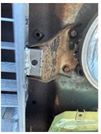
Check alignment of Grille AF in opening of truck – adjust as necessary so it is centered side to side as well as up & down.
