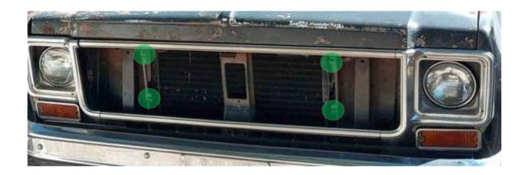
Remove headlight bezels on both sides of truck (5 Phillips head or Torx screws per size)
