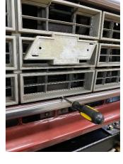
Install new plastic mounting tabs in the four locations below (only these four)
