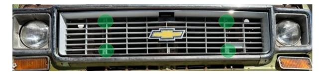
Install pan head screws in center top & bottom locations with washer & nutsert
