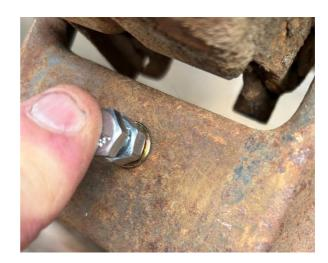
Using two wrenches, hold the bolt steady and tighten the nut until the nut-sert expands against backside of the hole.
