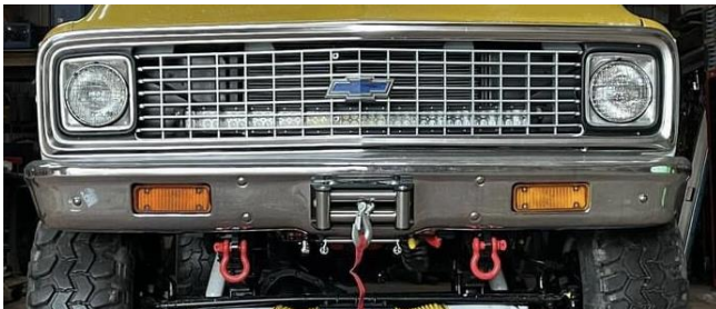
1972 K20 shown with BBWM in top mount configuration (winch cable through bumper) Also shown with Shackle Bracket Tow hooks (sold separately)
