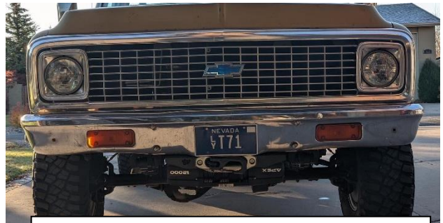
1972 K20 shown with BBWM in low mount configuration (winch cable under bumper)
