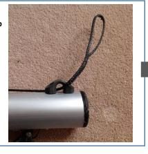
Step 2 – Pass the large loop through your clew block and back through the boom end eye. Then push the large loop over the end of the boom. Note that over time and use, the loop will tighten a bit as the line becomes softer.
