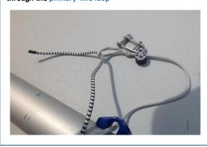
Step 5 – Pull the secondary line and the floating block all the way through the primary line loop until it looks like the photo below
