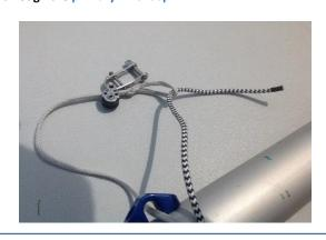
Step 5 – Pull the secondary line and the floating block all the way through the primary line loop until it looks like the photo below
