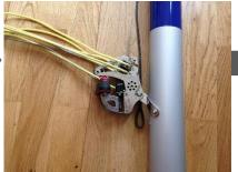
Step 3 – Pass the eye on the end of the small assembly through the primary line loop.
