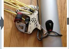
Step 6 – Thread the coloured control line from the block at the sail through the block at the kicker tang and back up to the block at the sail.
