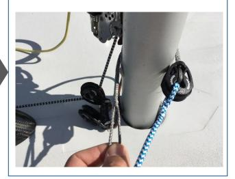
Step 4 – Thread the end of the secondary control line and the block through the loop on the lower block assembly strop.
