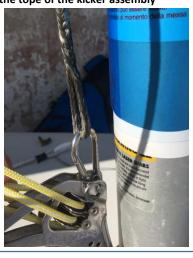
Step 3 – Pass the lower block assembly strop around the mast under the kicker tang
