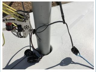
Step 3 – Pass the lower block assembly strop around the mast under the kicker tang
