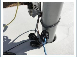
Step 5 – Route the secondary control line through the three blocks – it should look like the photos below.
