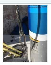
Step 3 - Pass the lower block assembly strop around the mast under the kicker tang and thread the block through the loop.
