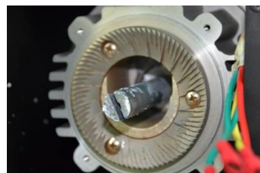
Step 9 – remove the disk holder
