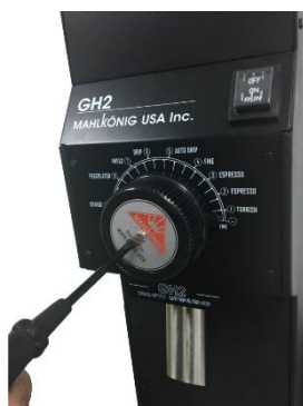
Fig 8-2 loosen the securing screws
