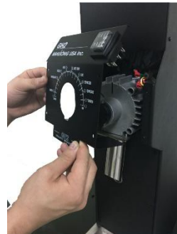
Step 3-mark and disconnect wires
