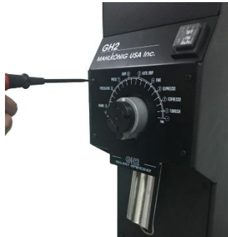
Step 2 – remove front cover step
