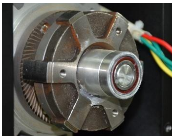
Step 7 –remove the bearing cover
