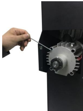
Step 5 – release grinding house
