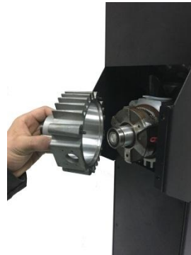
Step 6 -remove grinding house
