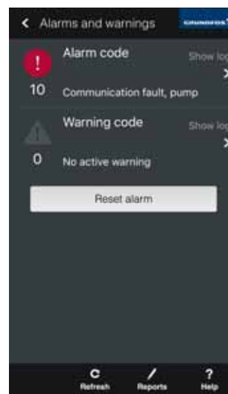
Fig. 33 "Alarms and warnings" menu with alarm
