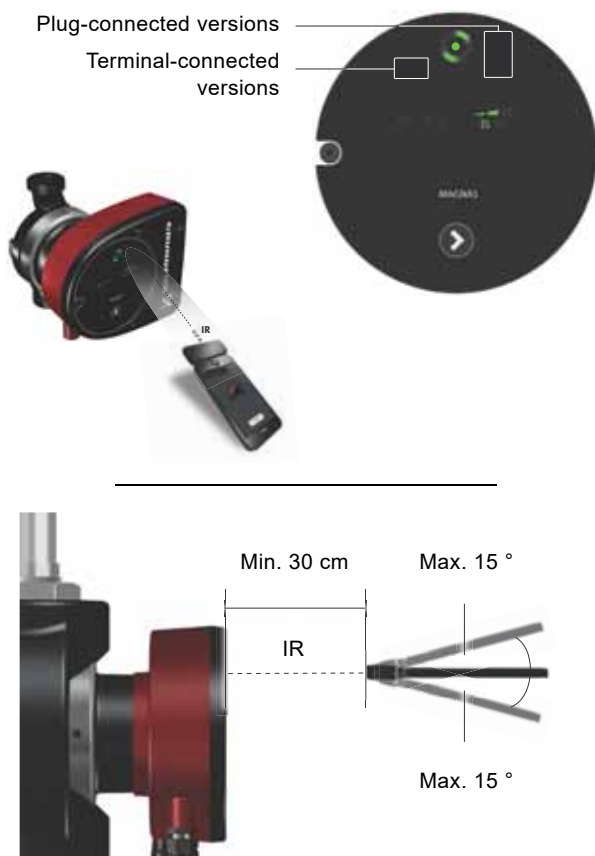
Fig. 29 Establishing a connection between Grundfos GO and MAGNA1 via infrared communication
