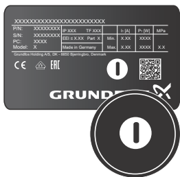
Fig. 36 Identifying the master pump head on the nameplate
