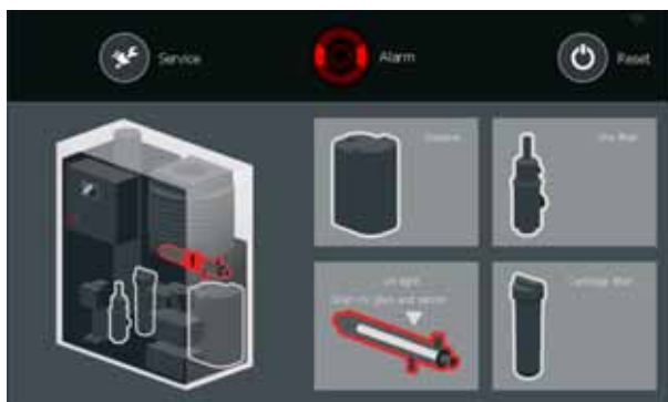
Fig. 16 Alarm indication - UV intensity sensor failure
