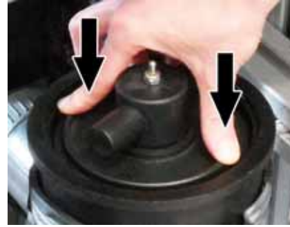
Fig. 21 Inserting the cyclone system
