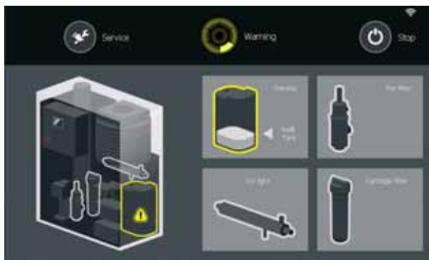
Fig. 15 Warning indication - low level in chlorine tank
