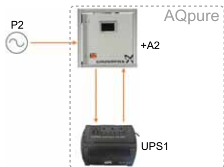
Fig. 11 AQpure system with UPS
