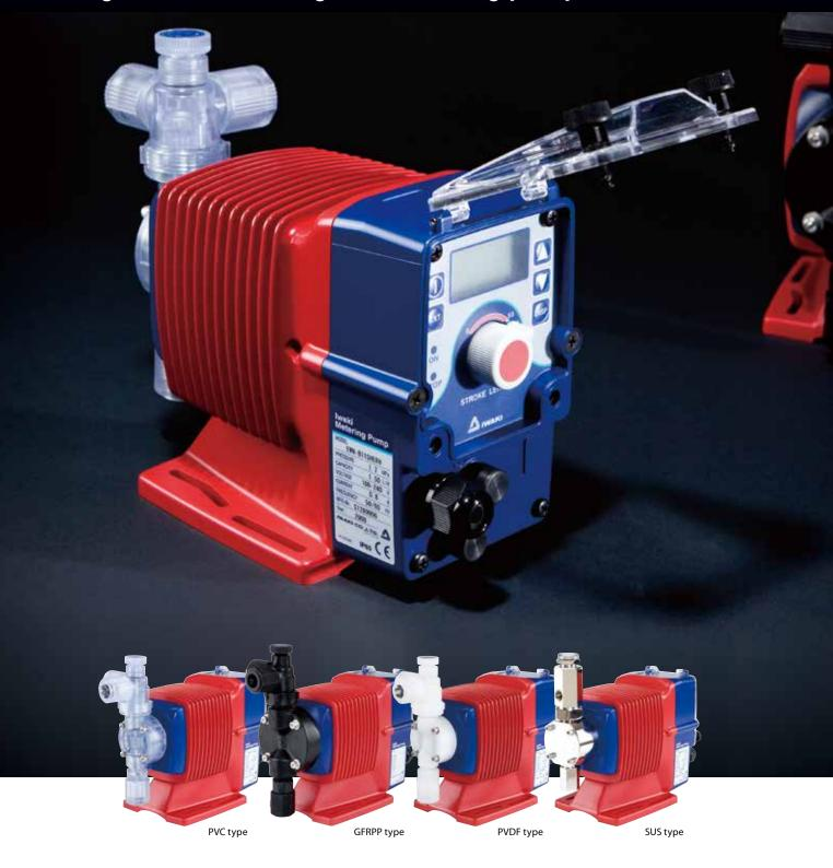
The EWN-R is the diaphragm type electromagnetic metering pump with a built-in multifunctional digital controller. Our technology makes the high-speed operation of 360spm available. The built-in controller that handles both digital and analogue signals controls operation in various ways. PVC, GFRPP, PVDF or SUS316 pump head is selectable. Also, special pump types for particular purposes are lined up. The user-friendly EWN-R will meet a wide variety of demands for chemical feeding.
