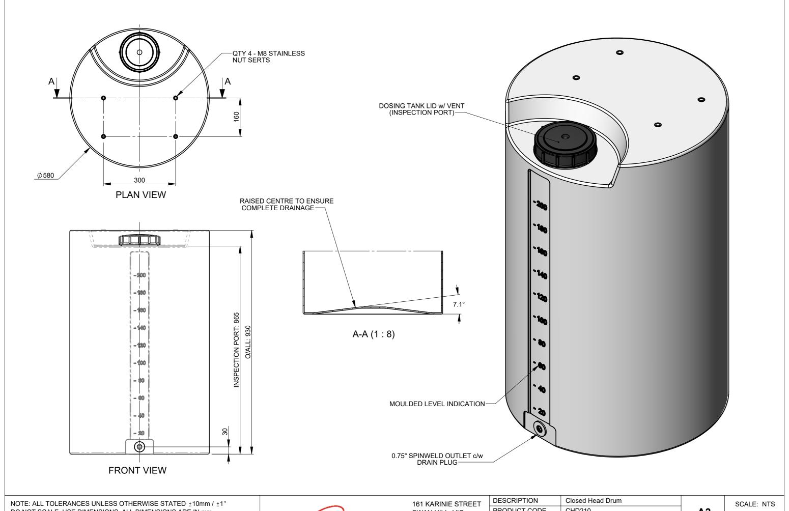
DO NOT SCALE, USE DIMENSIONS. ALL DIMENSIONS ARE IN mm
