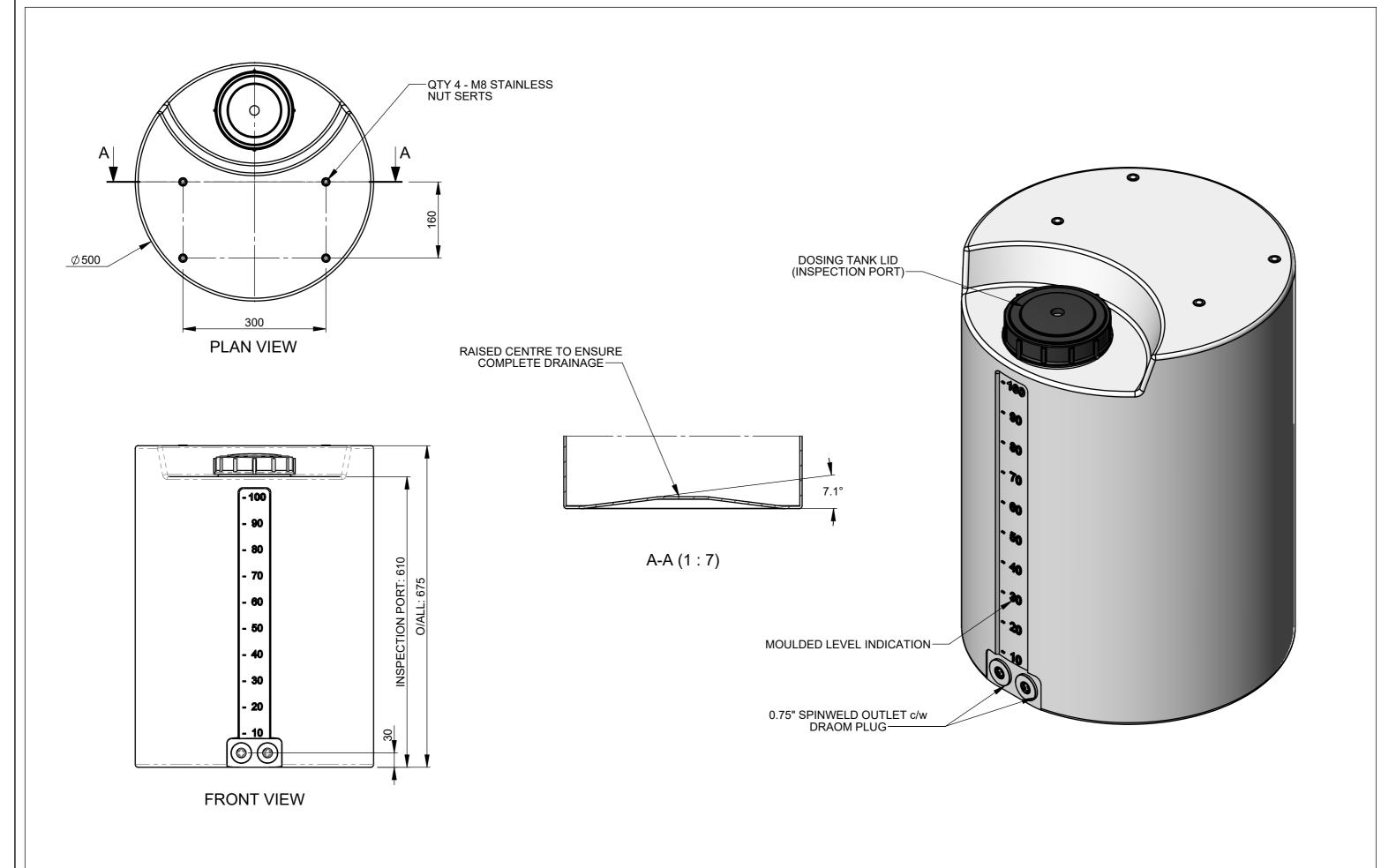
NOTE: ALL TOLERANCES UNLESS OTHERWISE STATED  $\pm 10$ mm /  $\pm 1^{\circ}$ DO NOT SCALE, USE DIMENSIONS. ALL DIMENSIONS ARE IN mm
