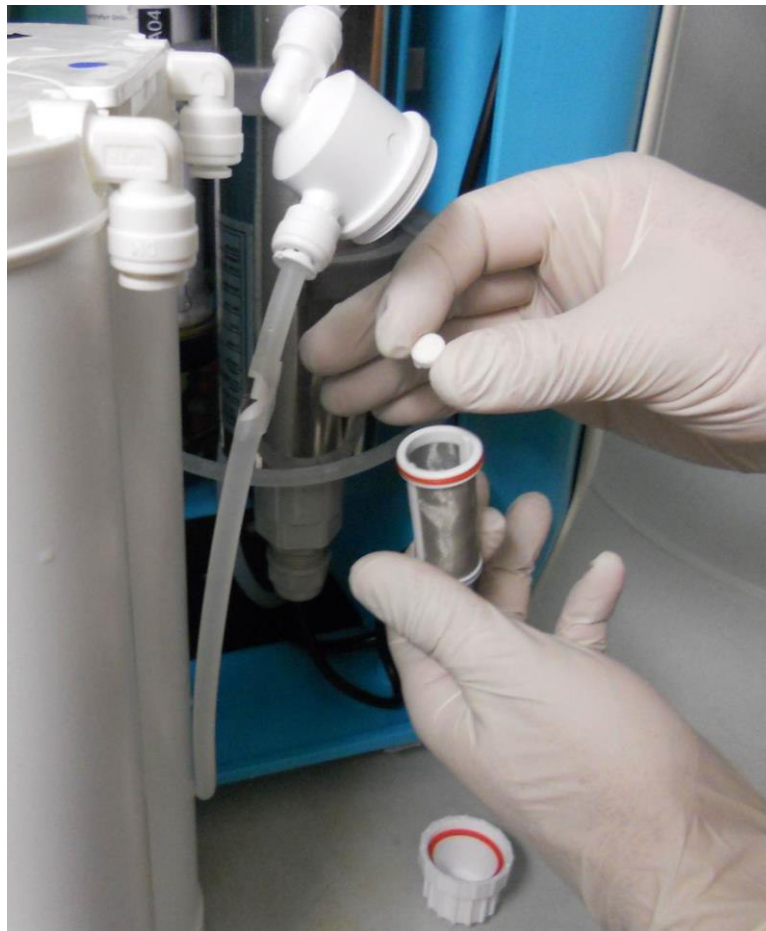
Figure 16: Opened disinfection cell
