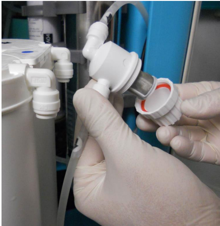
Figure 21: Disinfection cell with mounted strainer
